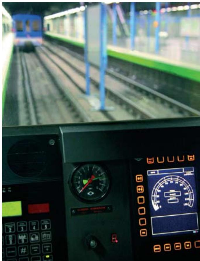
EBI Cab ATC onboard equipment
