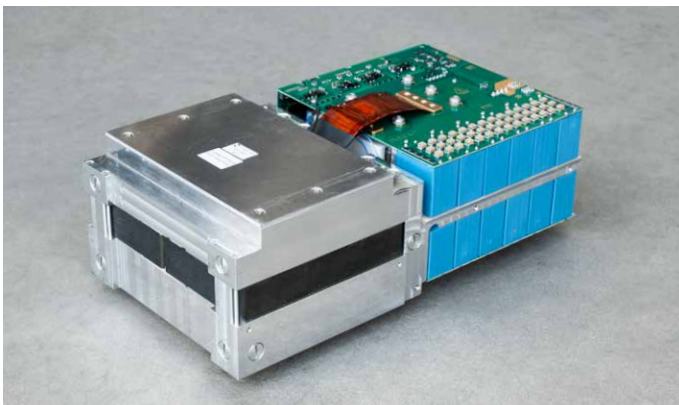
DC/DC converter with silicon carbide technology
